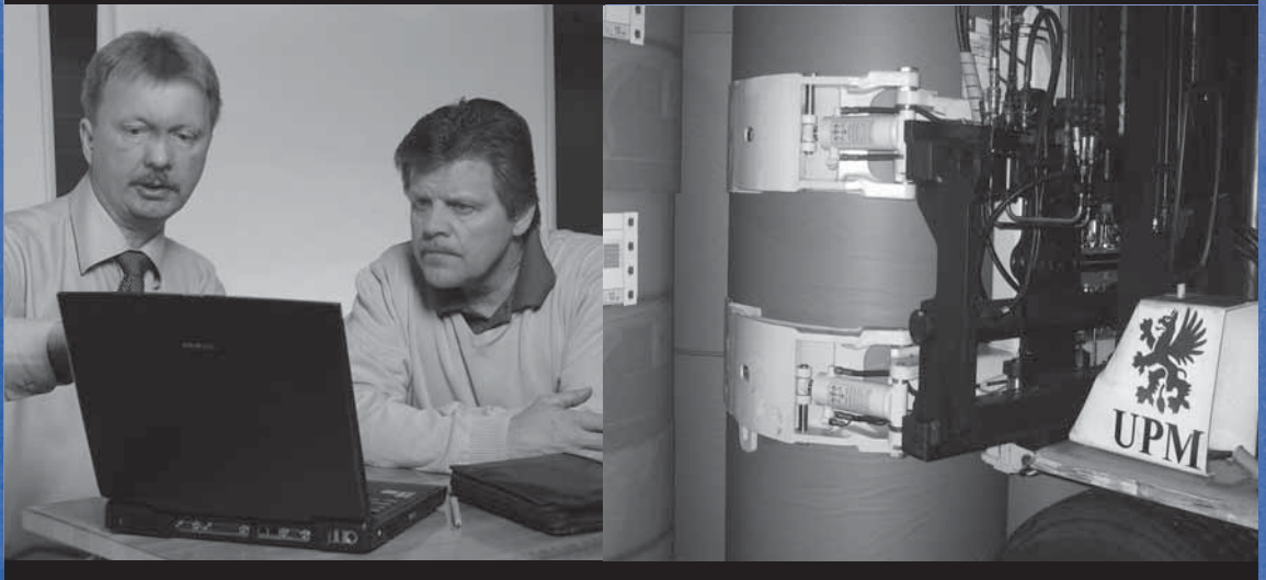
Right: Risto Miinin and Cascade's Tommy Abrahamsson discuss supply chain challenges Far Right: Double Tower clamp with Adaptive Force Control, installed on truck
