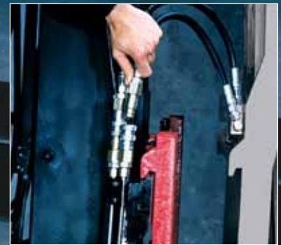
3. Connect quick-change hydraulic couplers
