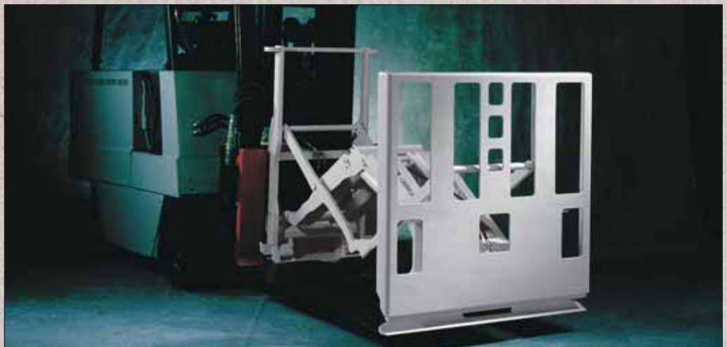
4. QFM Push/Pull is now ready for slipsheet loads.
