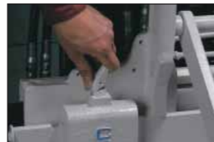
Platens are hung like conventional forks so spacing can be adjusted in seconds (carriage mount models).
